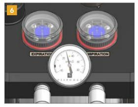
Check the manometer. The pressure must not drop (But it can increase). If the pressure drops, replace the patient circuit and the bag and try again.
