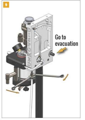
Install the oxygen supply hose to the back of the unit using 2 wrenches (5/8 and 11/16) in order to reduce the risk of accidentally disconnecting the hose.
