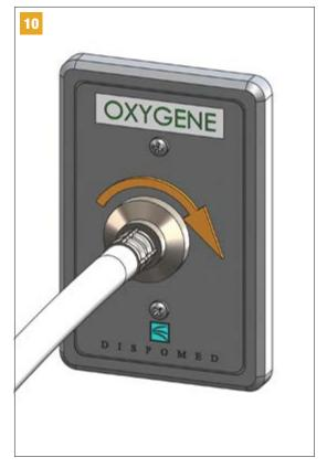
Connect the other end of the oxygen supply hose to a 50 p.s.i. (3 bar) oxygen supply.
