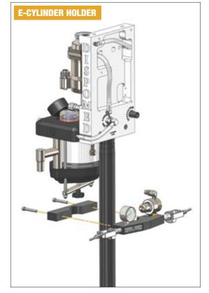
Installation of dual cylinder holder.
