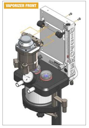
connect inlet-outlet fittings onto the vaporizer manifold.
