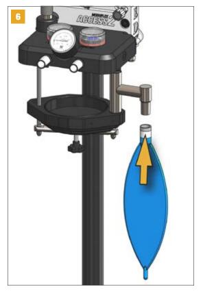
Install the vaporizer as indicated on page 12. Install a breathing bag on the rotary bag mount of the absorber.
